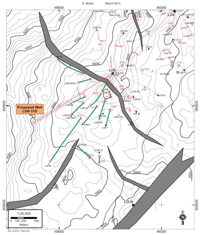
Fig. 1. Structural Map of Rio Bravo, showing the Proposed Well LO6-31D
